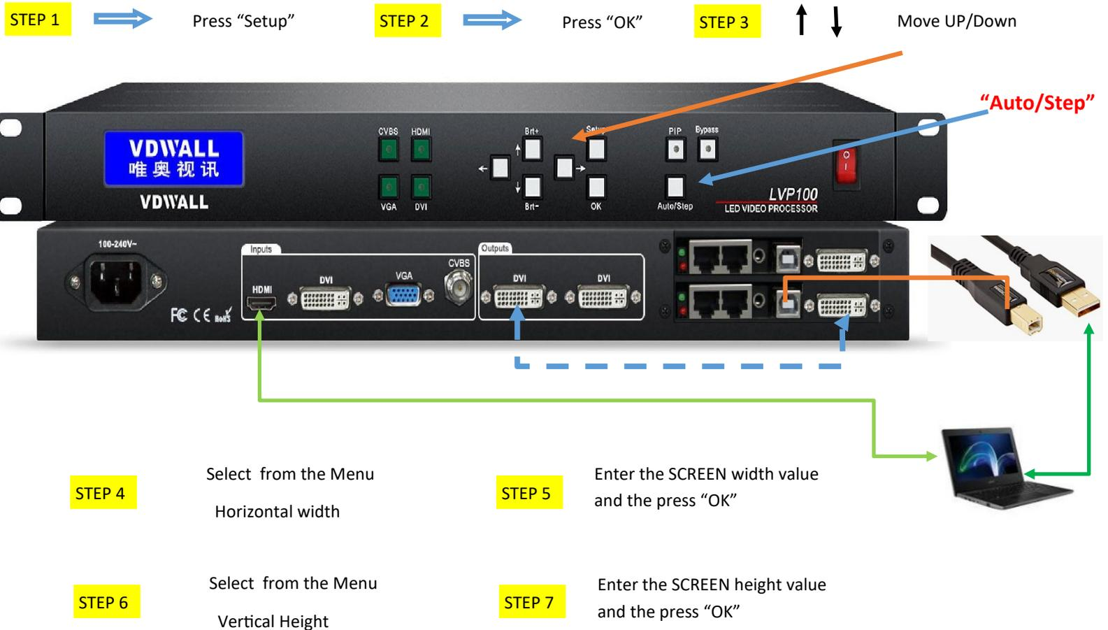
*NOTE : sometimes the step value don't coincide with the Screen Size , then use the "Auto/Step" button and select Step 2 in the Menu , this will allow to get the right number*
