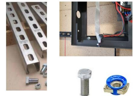
Struts will be mounted using 3/8 Bolts and 3/8 struts wing nuts , then cabinets will be secured to one another using 3/8" nuts and bolts
